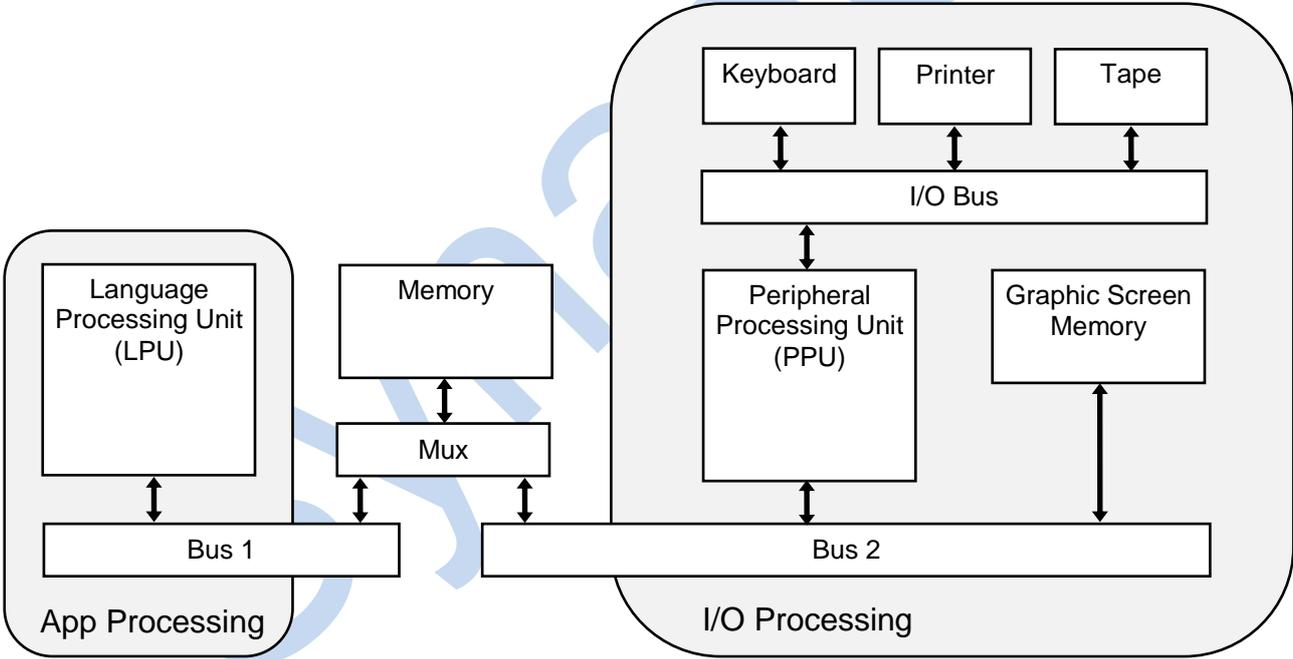
Fig. 3 - The first “workstation” principal construction
