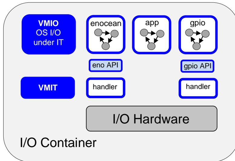
Fig. 7 - The basic software set for IoT device
